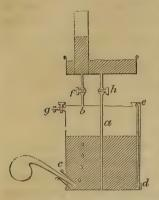
gas which is in constant requisition. It is usually made of japanned copper, and consists of a close cylindrical vessel, surmounted by a circular trough of the same diameter, but comparatively of small depth; a pipe a, proceeds from the bottom of the trough, and passing through the top of the air-chamber, descends until near the bottom, where it terminates in an open extremity. A second pipe, b, also passes down-
